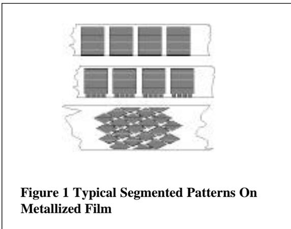
**Figure 1 Typical Segmented Patterns On Metallized Film**
