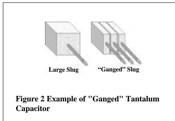
**Figure 2 Example of "Ganged" Tantalum Capacitor**
