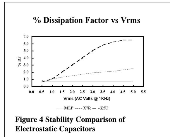
**Figure 4 Stability Comparison of Electrostatic Capacitors**
