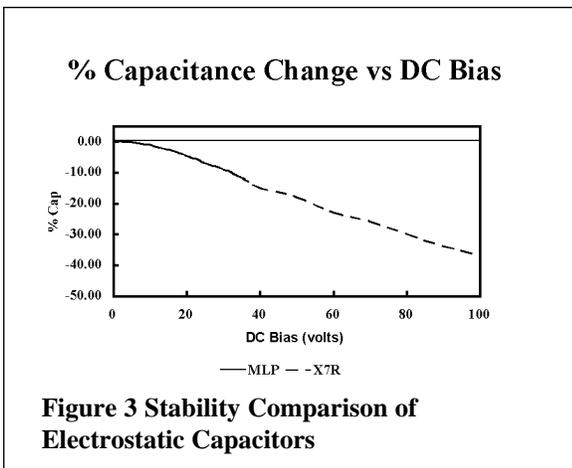
**Figure 3 Stability Comparison of Electrostatic Capacitors**
